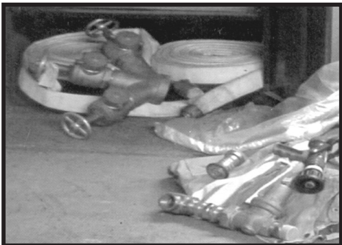
Example of manifolds, fire hoses, and nozzles commonly used
